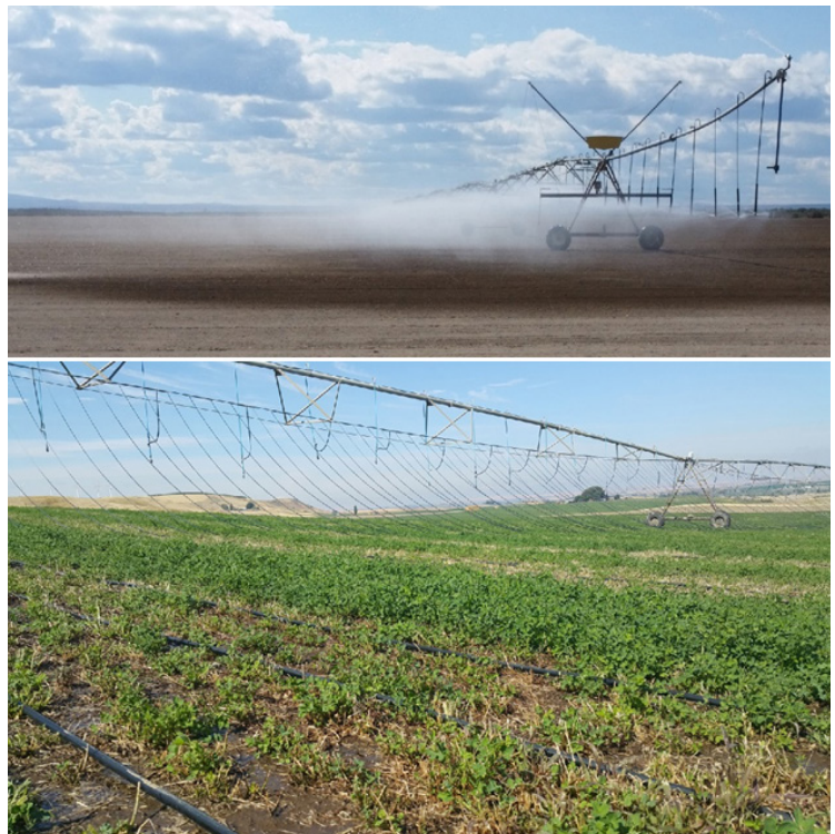
Center Pivot Sprinkler System (top) and Center Pivot System fitted with Mobile Drip Irrigation in an Alfalfa Field (bottom) Photo credit: Barber et al. 2020
